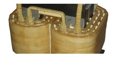
Special winding features developed by ABB allow a complete protection of the windings from water. Some customers have stretched us till the **5 kV applied** insulation test while the components are immersed in water.
