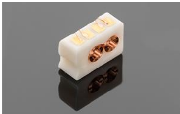
Custom micro-coil assembly Length 4mm, Coil \varnothing 1.2mm
